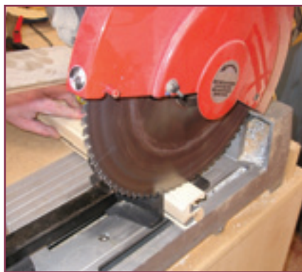
1. Cut Swan Systems Stiles to length using a chop saw.
