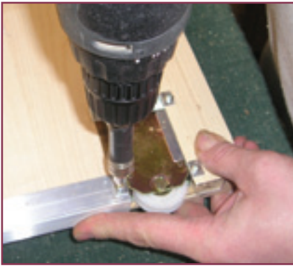
13. Attach the wheel housing and bottom aluminium rail, first by using 3mm drill bit, then 6/16" dome head flange screws.
