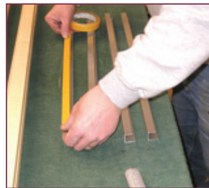
3. Using double sided adhesive tape, tape up the front of the top and bottom aluminium rails. The front of the rail is the SHORTER.
