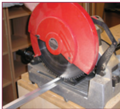
2. Cut Top and Bottom Ali Rail to length using a chop saw.
