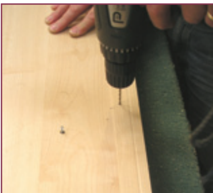
10. Using a 3mm drill bit, drill 4 holes at equal spaced intervals up the side stile.
