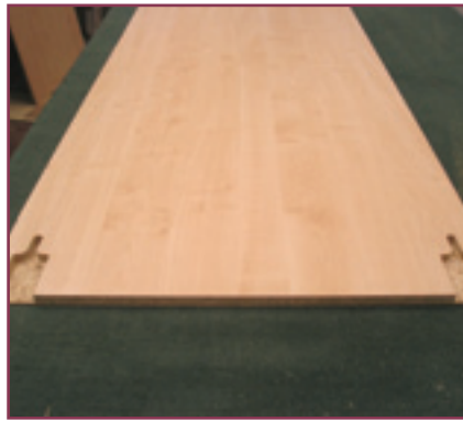
8. Repeat at the bottom left of the panel. Routing complete. Lift the panel and slide the carpeted batons under the panel, still face down.
