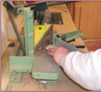
16. Using a Guillotine, cut square one end of the 55mm trim for the bottom of the door.
