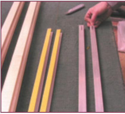
4. Apply two pieces of cut cushion pile to the back of the TOP aluminium rail, one to the left & right.
