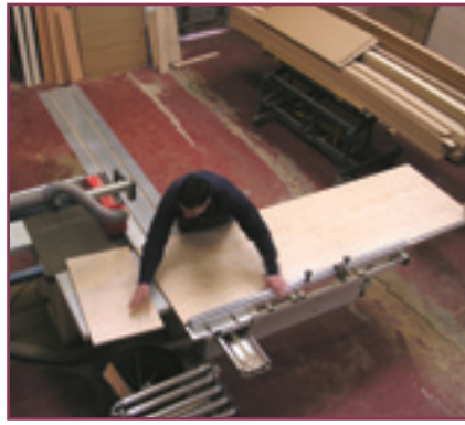
5. Set all these items to the side while you cut your panel to size.
